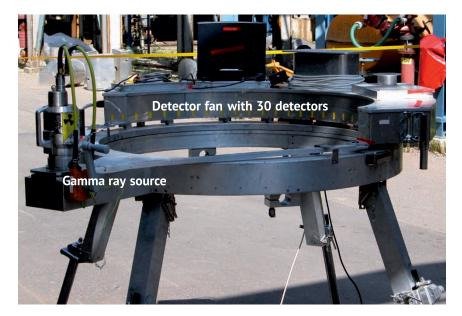
Computertomography at a 10" feed pipe of an upflow hydrogenating reactor for hydrocarbons
