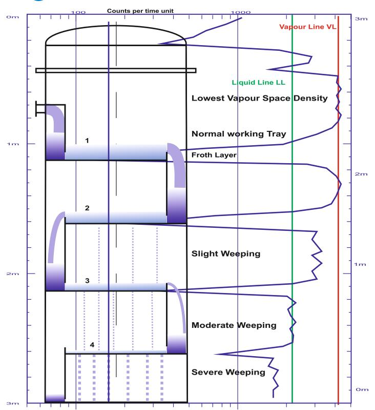
The weeping rate depends on vapour velocity, vapour cross flow area, liquid rate / weir height, tray type, seal of tray section overlap and manufacturing quality of trays. Possible reasons for weeping:
